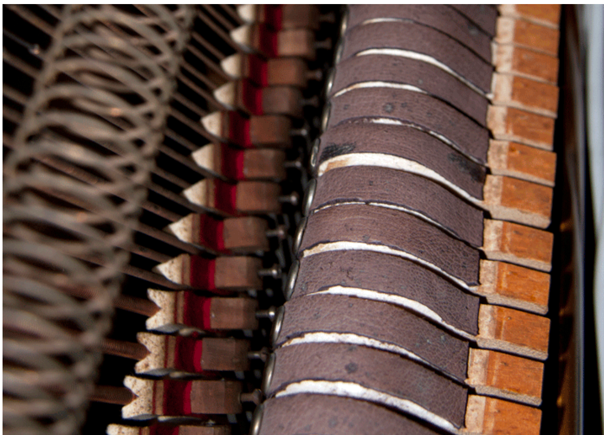
Figure 2. Nancarrow's piano with tacked hammers (picture by the author)
